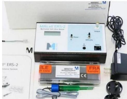
Millicell® ERS-2 Voltohmmeter (Millipore, Billerica, MA)
