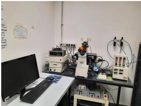
Fluorescence microscope with automated stage for multiple stage position XY and Z axes and with Okolab system for in vivo acquisition of cultured cells. MetaMorph Software.
