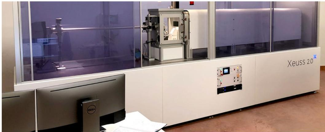
Fig.1: The Xenocs Xeuss 2.0-Q-Xoom diffractometer of SAXSLab Sapienza (room 058, building CU014)
